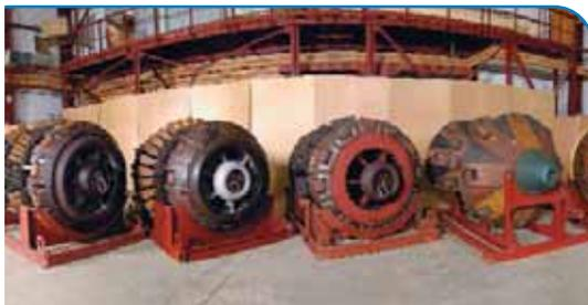
The complex of intrapipeline defectoscope produced by ZAO NPO "Spetsneftegaz" with the caliber of 1,400 mm.
