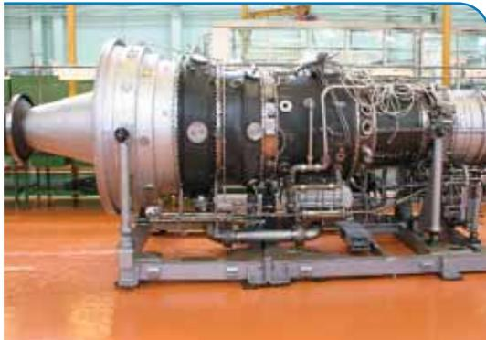
Drive Engine AL-31ST produced by OAO NPO "Saturn". Gazprom has established a technological base for the comprehensive reconstruction. It created and installed new types of gas pumping units at the compressor stations with efficiency up to 35 %.
